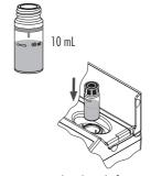
Press the Zero key. The display will show "-0.0-" when the meter is zeroed and ready for measurement.
