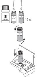
Press the Zero key. The display will show "-0.0-" when the meter is zeroed and ready for measurement.
