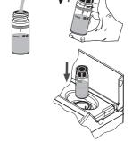
• Press **Timer** and the display will show the countdown prior to the measurement or alternatively, wait for 1 minute and press **Read**. When the timer ends the meter will perform the reading. The instrument displays the results in **mg/L** of chlorine (Cl<sub>2</sub>).
