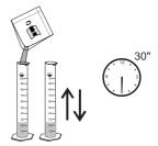
• Fill a cuvette with 10 mL of the reacted sample (up to the mark) and replace the cap.
