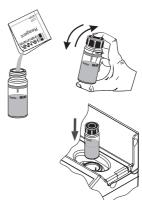
Press Timer and the display will show the countdown prior to the measurement or, alternatively, wait for 2 minutes and 30 seconds and press Read. When the timer ends the meter will perform the reading. The instrument displays the results in mg/L of bromine (Br<sub>2</sub>).
