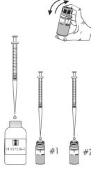
• Add 0.5 mL of HI93753B-0 Chloride Reagent B to each cuvette using the second 1 mL syringe.
