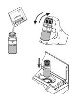
• Reinsert the cuvette into the instrument and close the lid.
