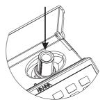
6. The meter is ready for use with 16 mm vial parameters. Always use the vial adapter for both "Zero" and "Read" measurements as specified in the parameter instructions.
