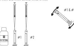
• Add one packet of H193738B-O Chlorine Dioxide Reagent B to one of the two cylinders (#1), cap and invert it several times until it is totally dissolved. This is the blank.
