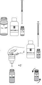
• Place the cuvette into the holder and close the lid.
