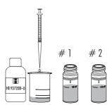
• Add 1 drop of HI93720C-O Calcium Hardness Reagent C to one cuvette (#1).
