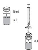
Insert the apparent color cuvette (#2) into the instrument and close the lid.
