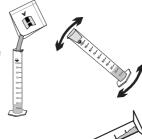
• Fill a cuvette with 10 mL of the reacted sample (up to the mark) and close the cap.
