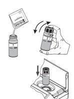
• Reinsert the cuvette into the instrument and close the lid.
