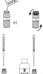
• Add 0.5 mL of HI96773B-0 Oxygen Scavengers Reagent B to each cuvette using the 1 mL syringe.
