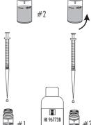
• Add 0.5 mL of HI96773B-0 Oxygen Scavengers Reagent B to each cuvette using the 1 mL syringe.
