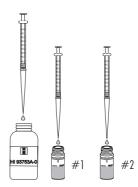
• Replace the caps and mix each cuvette by inverting for approximately 30 seconds.
