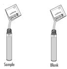
• Add 0.5 mL of deionized water to the first vial (#1, blank) and 0.5 mL of sample to the second vial (#2, sample), while keeping the vials at a 45-degree angle.
