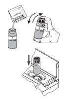
• Reinsert the cuvette into the instrument and close the lid.
