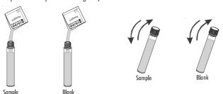
Press Continue and the display will show the countdown, or alternatively wait 2 minutes (without shaking the vials) to allow the reaction to complete.
