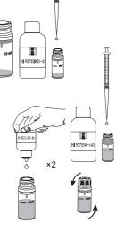
• Place the cuvette into the holder and close the lid.
