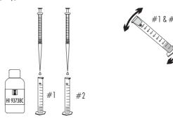
• Add 0.5 mL of H193738D-0 Chlorine Dioxide Reagent to each cylinder (#1 & #2), using a 1 mL syringe, cap and invert several times to mix. Cylinder #2 is the reacted sample.
